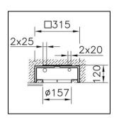
Weight 2.45 kg Embedding housing B.Box for fairced concrete, in steel, sendzimized,
