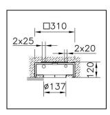
Weight 2.15 kg Embedding housing B.Box in steel sheet, sendzimized, round, opening  $\emptyset$  = 137 mm, EL = 310 mm, EB = 310 mm, ET = 120 mm,
