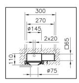
**Finish** grey Weight 0.06 kg Embedding housing B.Box in polyethylene (PE), grey, with control gear tank, without halogen, round,  $\emptyset$  = 145 mm, opening  $\emptyset$  = 75 mm, EL = 270 mm, ET = 110 mm,
