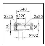
Embedding housing B.Box in synthetic material, with control gear tank, round,
