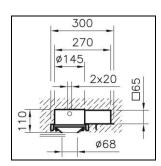
**Finish** grey Weight 0.5 kg Embedding housing B.Box in synthetic material, grey, with control gear tank, round,
