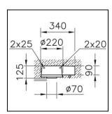
Weight 1 kg Embedding housing B.Box for fairced concrete, in polycarbonate (PC), with control gear tank, without halogen, round,  $\varnothing$  = 220 mm, opening  $\varnothing$  = 70 mm, EL = 340 mm, EB = 220 mm, ET = 125 mm
