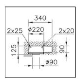
Weight 1 kg Embedding housing B.Box for fairced concrete, in polycarbonate (PC), with control gear tank, without halogen, round,  $\varnothing$  = 220 mm, opening  $\varnothing$  = 90 mm, EL = 340 mm, EB = 220 mm, ET = 125 mm
