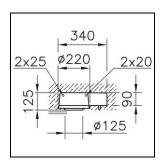
Weight 1 kg Embedding housing B.Box for fairced concrete, in polycarbonate (PC), with control gear tank, without halogen, round,  $\emptyset$  = 220 mm, opening  $\emptyset$  = 125 mm, EL = 340 mm, EB = 220 mm, ET = 125 mm
