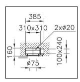
Weight 0.453 kg Embedding housing B.Box for fairced concrete, in polycarbonate (PC), without halogen, round, opening ø = 75 mm, EL = 385 mm, EB = 310 mm, ET = 240 mm
