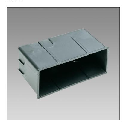
**Finish** black Weight 0.25 kg Recessed housing Megabrique S.4523 in synthetic material, rectangular black EL = 263 mm EB = 135 mm ET = 95 mm
