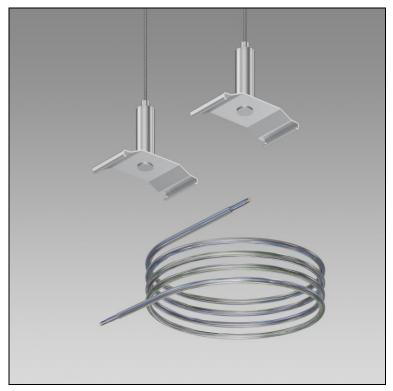
Weight 0.183 kg Suspension kit Purelite Slim with wire suspension and self-lock, recommended: every 1,5 m, 2 wire cords, clippable, with 1.8 m power connection cable, 5 poles, transparent, with cable clamp,
